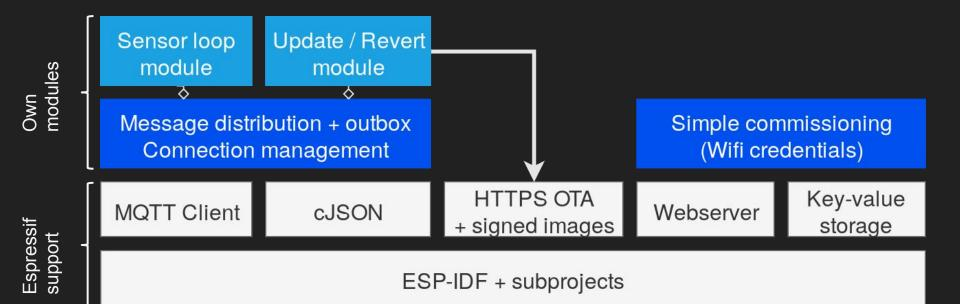
ESP-IDF: FreeRTOS with multi-core support adapted for ESP32
